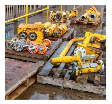
NORM scale is removed from contaminated equipment at the Tradebe Scotoil permitted facility in Aberdeen mainly by high and ultra-high pressure water jetting techniques.
